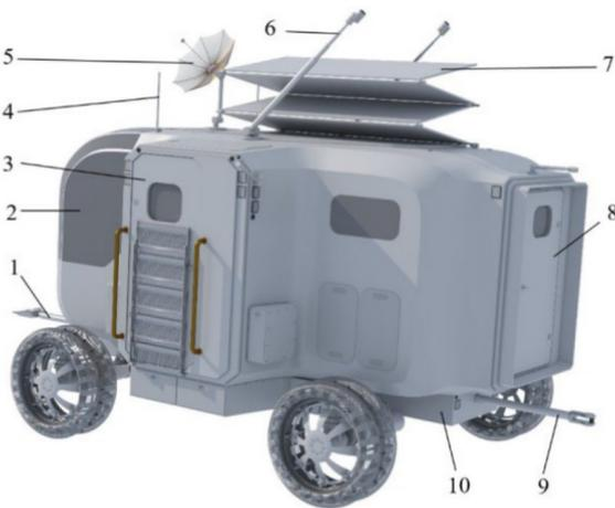
**Fig. 2.** Conceptual Design of the Head (Piloted) Link of the Lunar Train: 1, 9 — Active and passive parts of the ADCU; 2 — Cabin windshield; 3 — Airlock chamber for surface access; 4 — Pin antenna; 5 — Highly directional antenna; 6 — Panoramic camera (in deployment); 7 — Solar panel (in deployment); 8 — Airlock chamber for docking with the second link of the lunar train; 10 — Self-propelled chassis of the IMP
